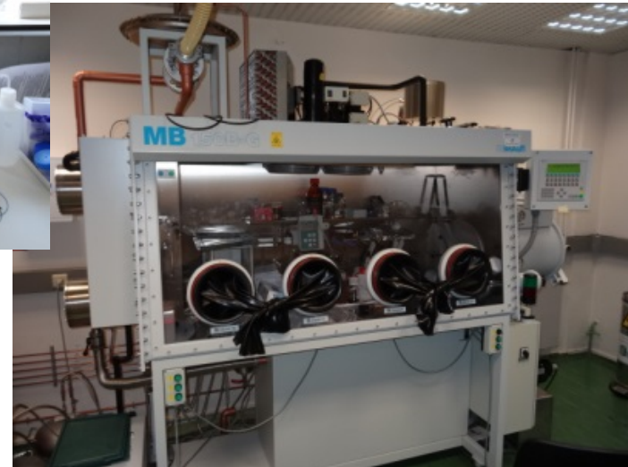
Glove boxes for working under controlled (anoxic) atmosphere
