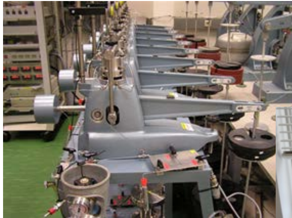
Oedometer setups for swelling behaviour of Eurobitum
