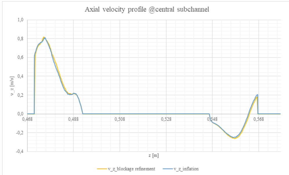
Figure 51 – Effect of the inflation layer on the velocity profile along the line at the centre of the blocked subchannel in the refined blockage domain
