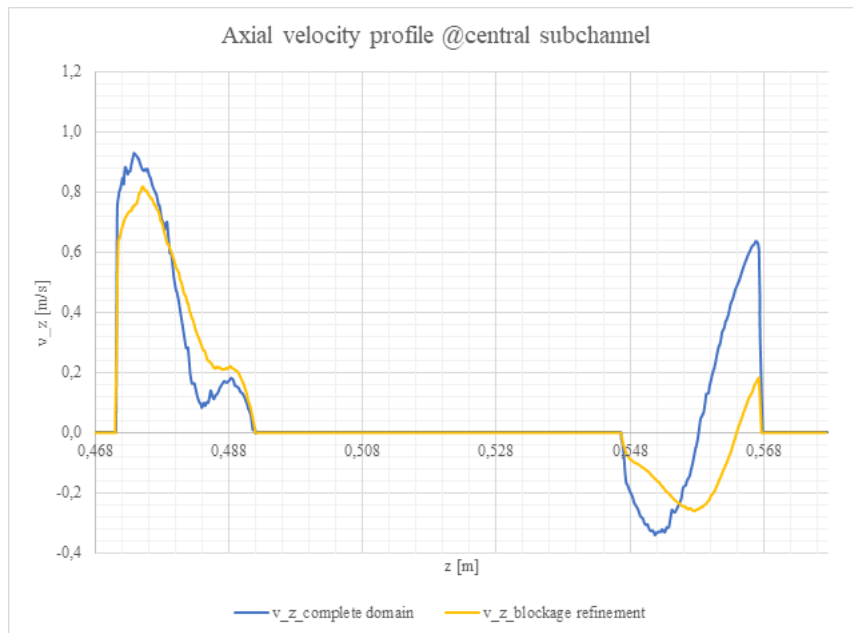
Figure 47 – Comparison of the velocity profiles along the line at the centre of the blocked subchannel between the refined blockage domain and the complete domain
