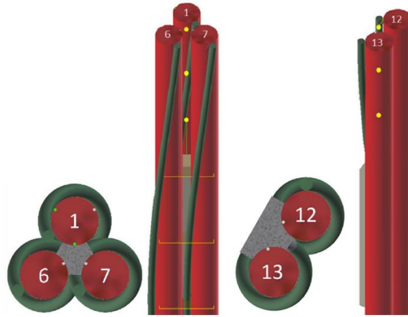
Figure 9 – Position of the thermocouples installed at the blockages mid-height and in the blocked subchannel in their wake region (C1 on the left and E1 on the right) [45]
