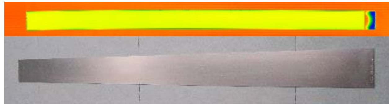
DU UMo monolithic plate ; Ultrasound picture (top); Visual picture (Bottom)
