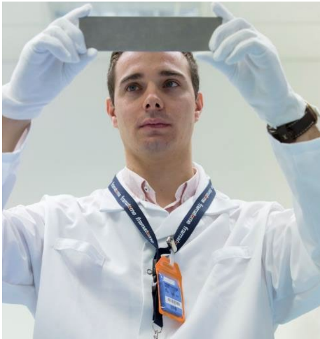
Medical target for Mo-99 production ~200 x 45 x 1.6 mm
