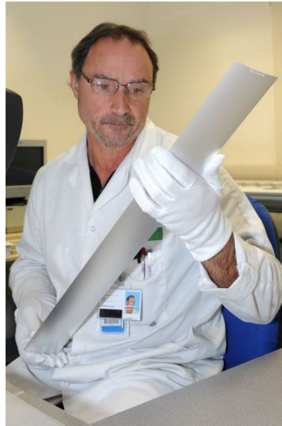
Fuel plates for Research Reactors ~600 x 60 x 1.3 mm
