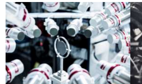
050: GELINA – time-of-flight facility Electron accelerator for neutron interaction measurements
